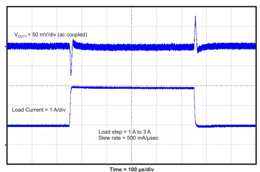
Figure 9. TPS54495EVM Converter 1 Load Transient Response
