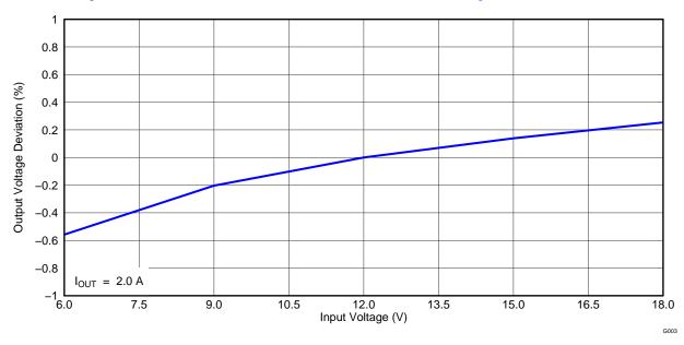
Figure 7. TPS54495EVM Converter 1 Line Regulation
