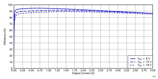
Figure 1. TPS54495EVM Converter 1 Efficiency
