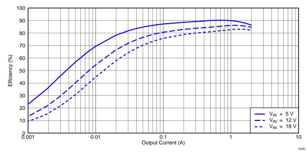
Figure 4. TPS54495EVM Converter 2 Light Load Efficiency
