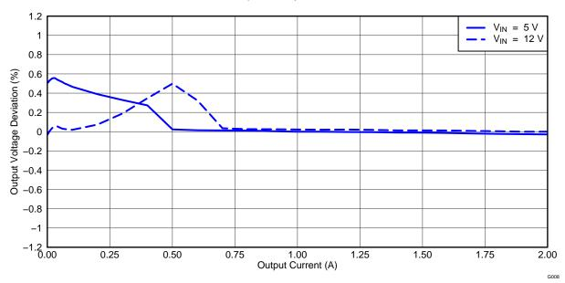
Figure 6. TPS54495EVM Converter 2 Load Regulation
