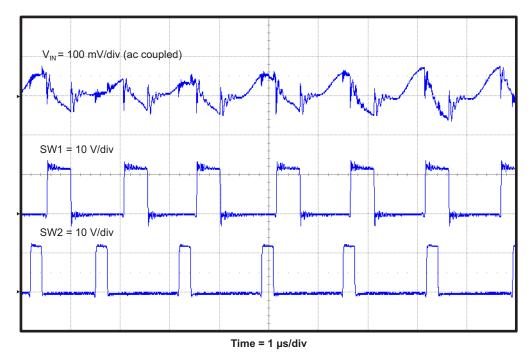
Figure 15. TPS54495EVM Input Voltage Ripple
