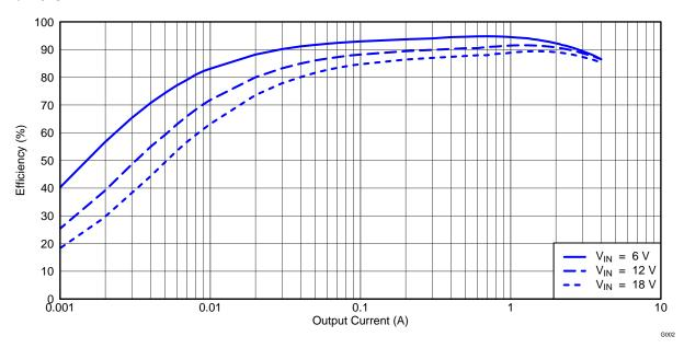
Figure 2. TPS54495EVM Converter 1 Light Load Efficiency
