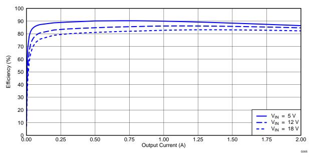
Figure 3. TPS54495EVM Converter 2 Efficiency
