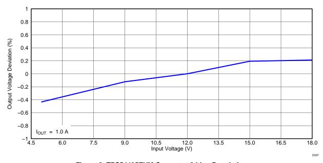
Figure 8. TPS54495EVM Converter 2 Line Regulation
