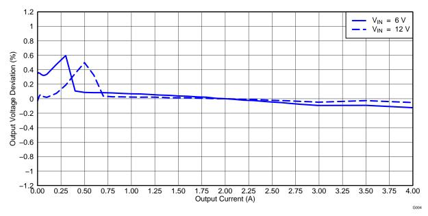
Figure 5. TPS54495EVM Converter 1 Load Regulation
