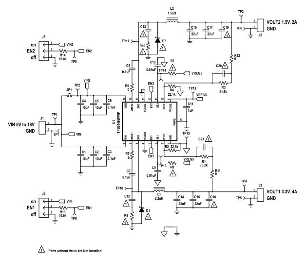
Figure 26. TPS54495EVM Schematic Diagram
